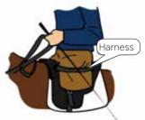
▲ Special harness The illustration shows a safety belt attached to the saddle, which is used for the riders' safety and is designed to come off immediately in case of danger.
